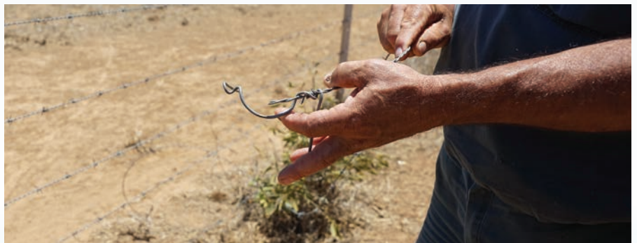
Broken wire: A multi-strand barbed wire fence is no match for determined kangaroos, who will push under the fence, spreading the barbs. The continual movement of the wire eventually causes it to wear through at the post.
