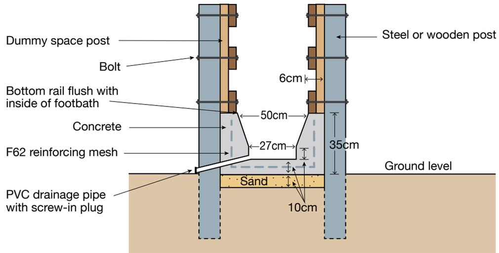
*Figure 4b: Main features of a walk-through footbath — elevation (not to scale)*
