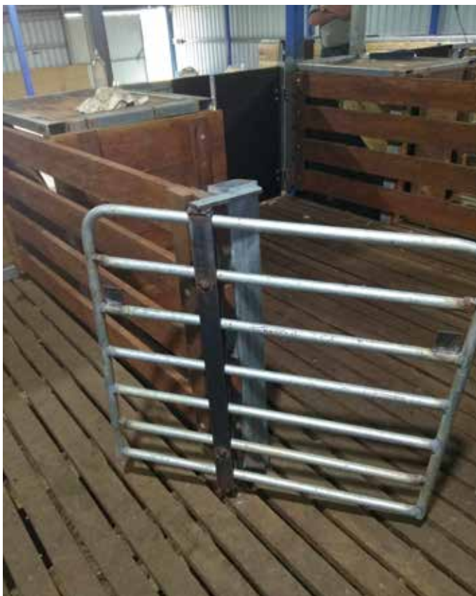
Figure 5: side fill catching pen with a slide/swing gate and boarded off chute to remove any trip hazard.
