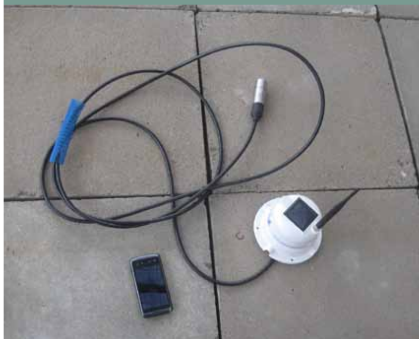
Figure 4: Smart Water telemetry system.
