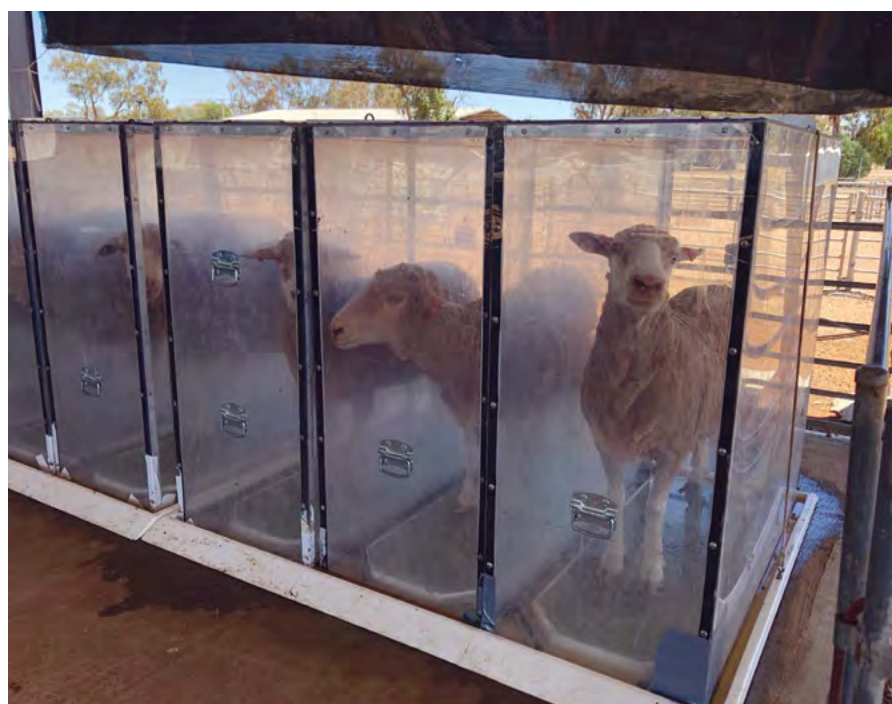
Macquarie MLP ewes in portable accumulation chambers to assess their methane emission rate.
