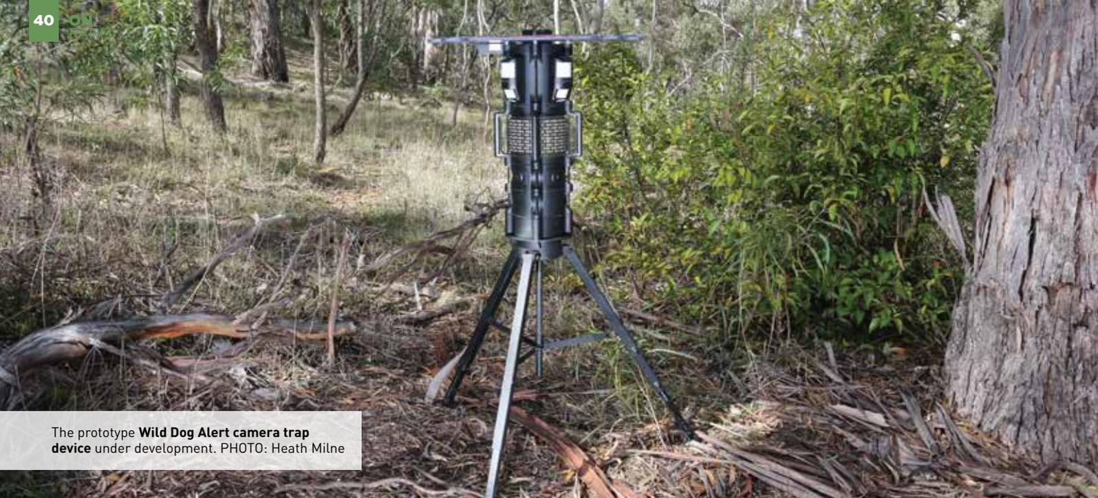
The prototype **Wild Dog Alert camera trap device** under development. PHOTO: Heath Milne
