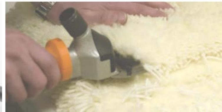
The belt-mounted drive system of this handpiece was developed, including a motor, battery and motor controller.
