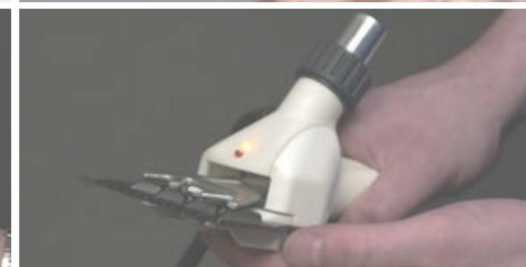
A new mechanism was developed that would allow the drive shaft to travel down the arm of the shearer and join the device where the cutter tensioner sits. This would also help to take some of the weight of the device, as the drive shaft would be above the handpiece rather than behind it.
