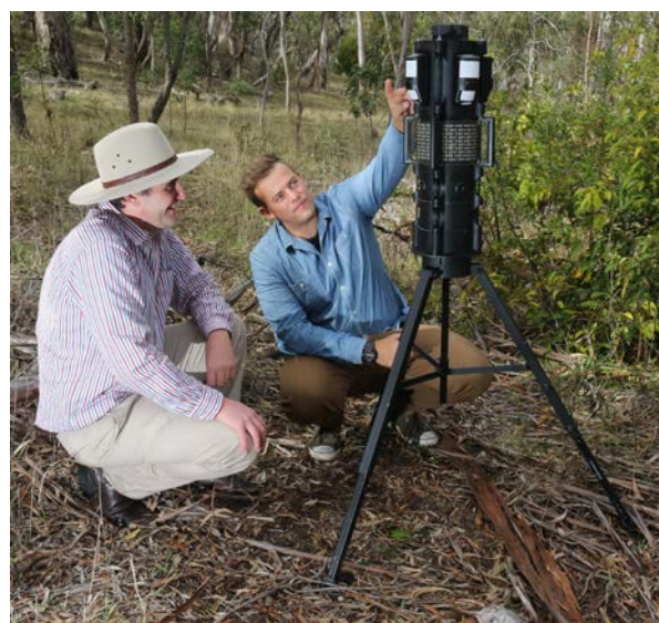
Using an automated on-property camera trap device that identifies wild dogs, the Wild Dog Alert system aims to notify a woolgrower of a wild dog's presence in real-time, to enable the woolgrower to act early.
