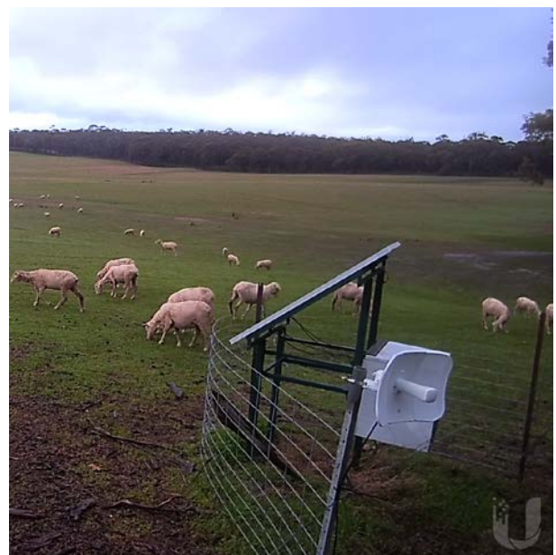
Vision from a camera on a wireless network at Tony Butler's property at Newstead, Victoria, also showing the point-to-point antenna (bottom-right) that is able to create reliable links over 20km line of site.
