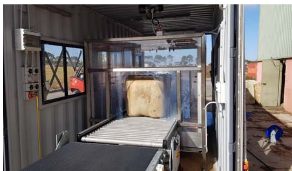
A prototype bale sprayer that aims to allow rapid disinfection of the outside of wool bales.
